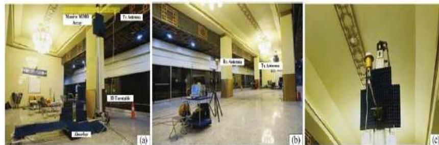
5G massive MIMO channel sounder, from 2 GHz to 26 GHz, with max. 160 MHz bandwidth and 256 elements
