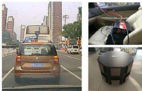
5G V2V/V2I channel sounder, including 2.6 GHz and 5.9 GHz, 3D antenna array with 32 elements
